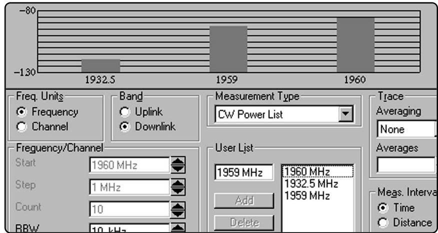
Figure 36. CW power measurements using the receiver-based solution are useful for the site evaluation stage of the wireless network life cycle. Channel power measurements are also available from this same user interface.
